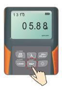
2. Press and hold the "REF" key over 2 seconds to store the presently measured value as the new reference level for the current wavelength. During the process the "REF" sign flashes twice on the screen and buzzer sound is heard. Once the new reference level is set, the FHP2 switches to the dB measurement mode. The displayed value only lasts 1 second.
